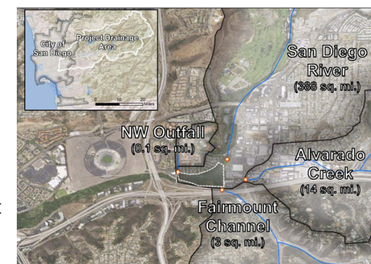
Map of the Project Site, Stream Inputs, and Their Corresponding Drainage Areas Source: TetraTech, 2017
