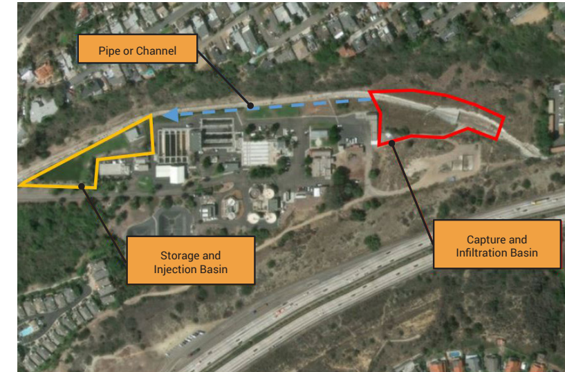
SEWRF Stormwater Capture Elements
